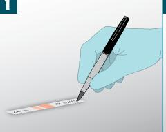
Remove a PINNACLE AEC test strip from bottle and, using a permanent marker, write the equipment identification, date, time and location, if applicable, on the strip handle.
