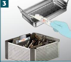
Securely attach the test device inside the **middle or lower instrument baskets** or on the **perimeter** of the washer-disinfector rack making sure there is no contact with the spray arm. For ultrasonic cleaners, **securely attach to instrument basket**.
